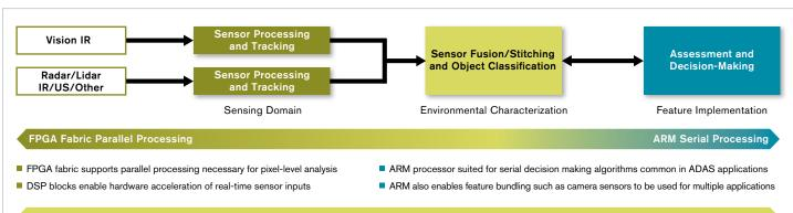
Idealized Hardware and Software partitioning becomes possible with FPGA/Processor Integration
