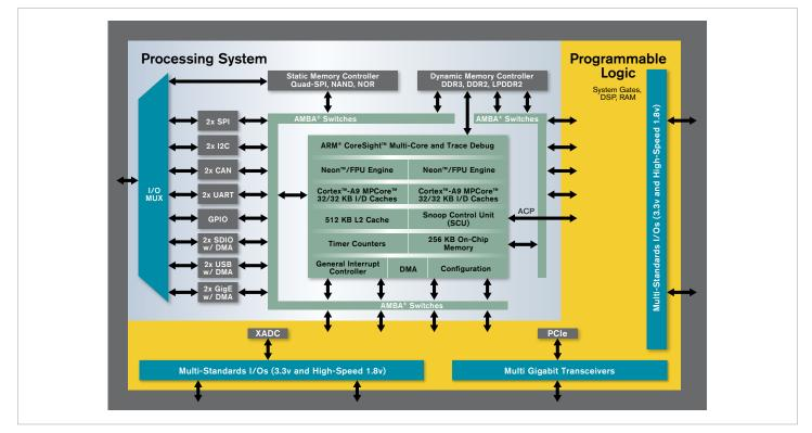
The software programmability of the dual-core ARM<sup>™</sup> Cortex-A9 processor is combined with the hardware programmability of FPGA logic. Large amounts of on-chip programmable I/O and AXI-based interconnects complete the All Programmable SoC, enabling unprecedented advanced design possibilities. Designers can accelerate complex image and video processing with the flexibility to support 360° surround view, blind spot detection, pedestrian sensing, lane departure warning and more.
