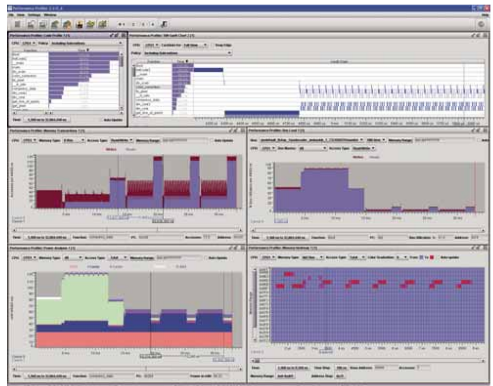
Figure 1 – Seamless FPGA's system profiler helps you tune performance by providing detailed data on bus transactions and utilization, software function execution time, bus arbitration delay, memory hot spots, and software code profiling.
