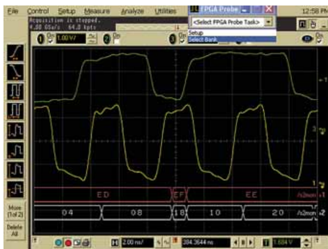
Figure 1 – In addition to scope channels, mixed-signal oscilloscopes provide 16 digital channels. This gives you the ability to trigger and display as many as 20 signals simultaneously. The width of the digital channels is particularly well suited for measuring signals internal to Xilinx FPGAs.
