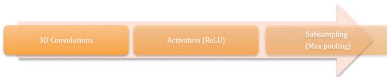
Figure 2 – A convolution layer in AlexNet does 3D convolutions, activation and subsampling.
