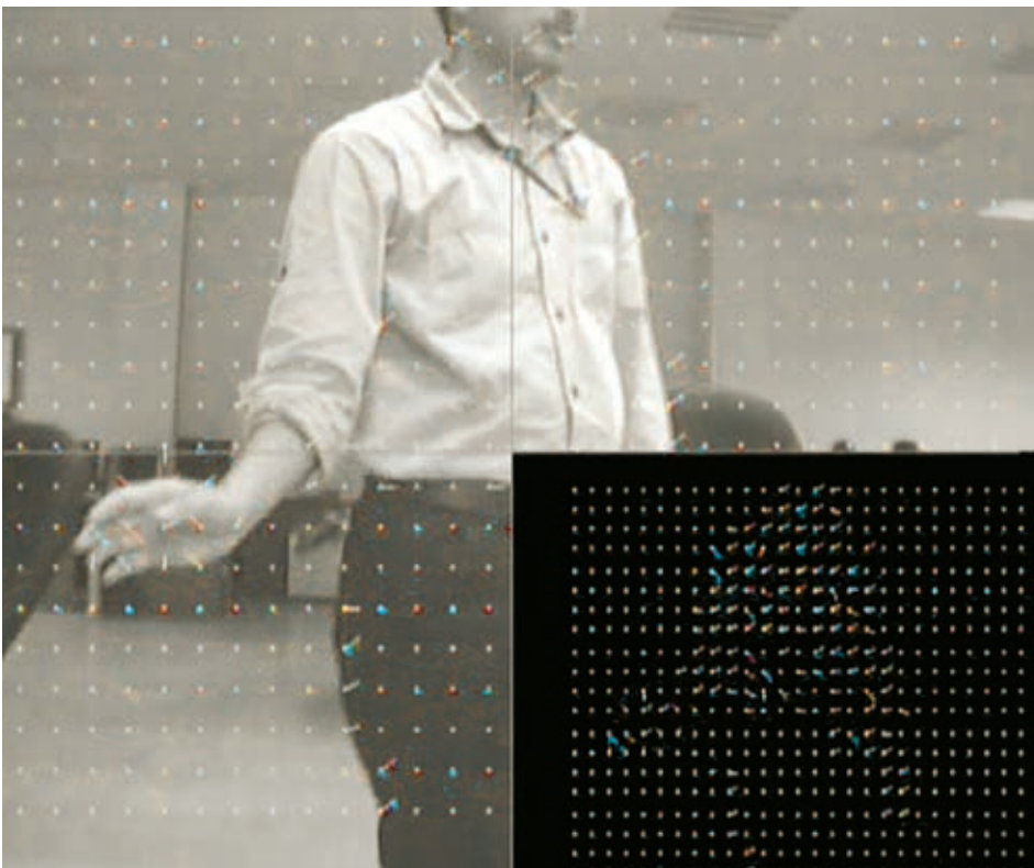
Figure 4 – An actual FPGA-processed frame with motion vector grid overlaid at bottom right
