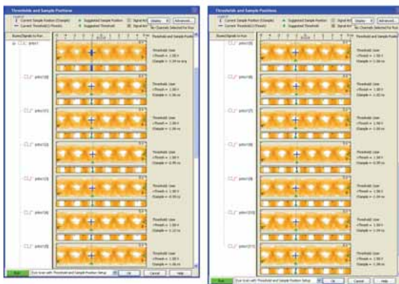
Figure 5 – EyeScan and EyeFinder view of all bits for 2x TDM core at 300 MHz
