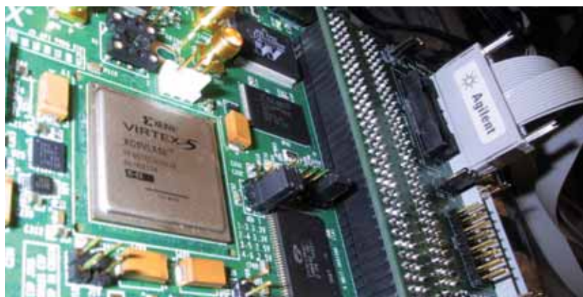
Figure 7 – Single-ended 1.5 Gbps SoftTouch connector-less probe connection to a Virtex-5 FPGA with ATC2 TDM core
