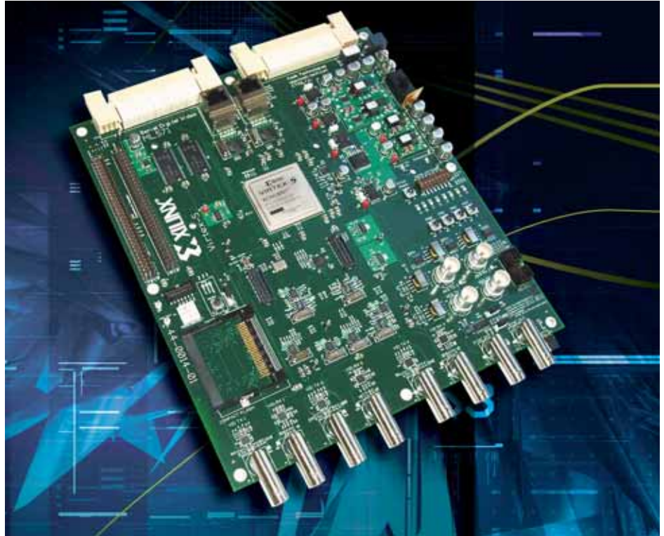
Figure 1 – ML571 board and frame synchronization demonstration board with an ASRC to match the output digital audio rate to the output digital video rate.
