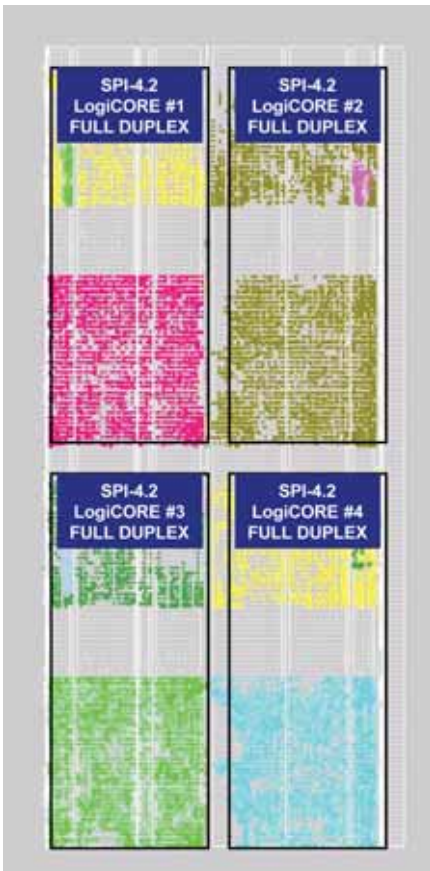
Figure 3 – Illustration of four instances of SPI-4.2 LogiCORE IP implemented on a Virtex-5 XC5VLX110 device
