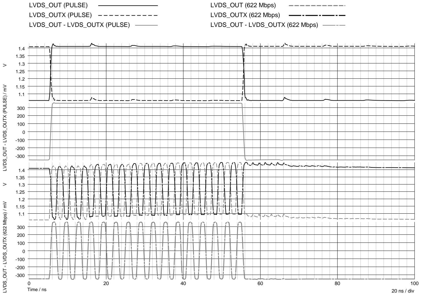
Figure 15: Pulse and 622Mb/s Burst Data Response of the Virtex-E LVDS Line Driver in Figure 2 with 5 ns Transmission Lines
