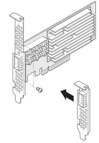
An optional 1PPS bracket and cable assembly, Solarflare part number SOLR-PPS-DP40G, is available for Solarflare QSFP+ server adapters. For detailed fitting instructions, refer to the *Solarflare Server Adapter User Guide*.
