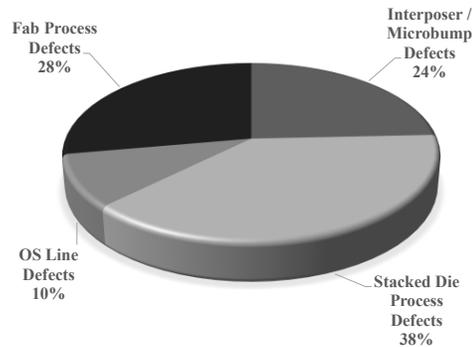
**Figure 10.** Failure Pareto (% of % Defects) for Assembly
