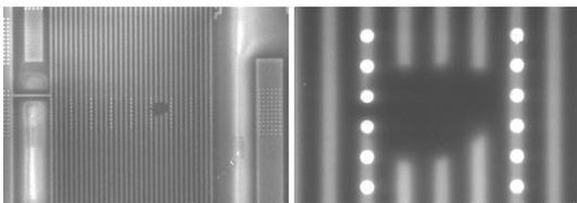
**Figure 5(a).** An Example of Interconnect Line Defect
