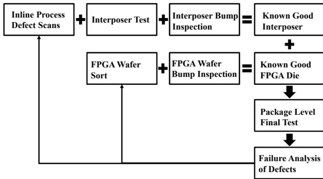
**Figure 4.** Continuous Yield Improvement Process Flow
