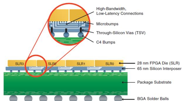
Figure 1. Schematic X-section of Virtex®-7 2000T FPGA Assembled with Interposer with TSVs
