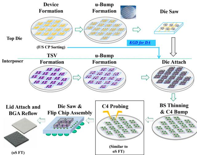
**Figure 9.** Process Flow with Additional C4 Probe Test Point
