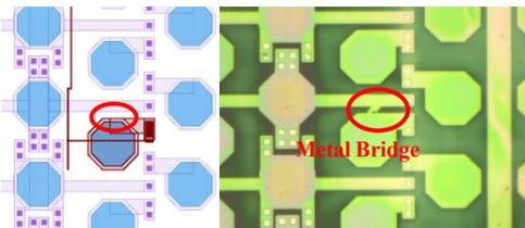
**Figure 5(c).** An Example of Metal Bridge in RDL Layer
