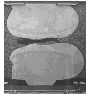
**Figure 6.** Example of uBump Open Caused by Contamination
