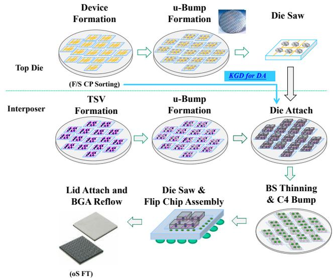
Figure 3. Simplified Package Assembly Process Flow
