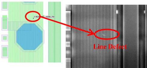
**Figure 5(b).** An Example of An Interconnect Line Defect
