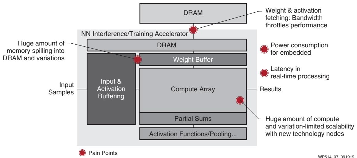
Figure 7: Typical “Pain Points” in a Generic DPU Architecture
