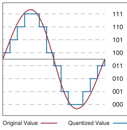
Figure 3: 3-Bit Quantization Function of a Sine Wave
