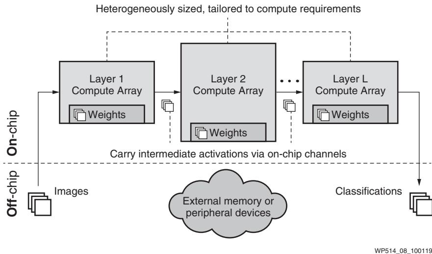
**Figure 8: FINN, a Soft DPU with Dedicated Per-layer Compute Resources and On-chip Data Flow between Layers**
