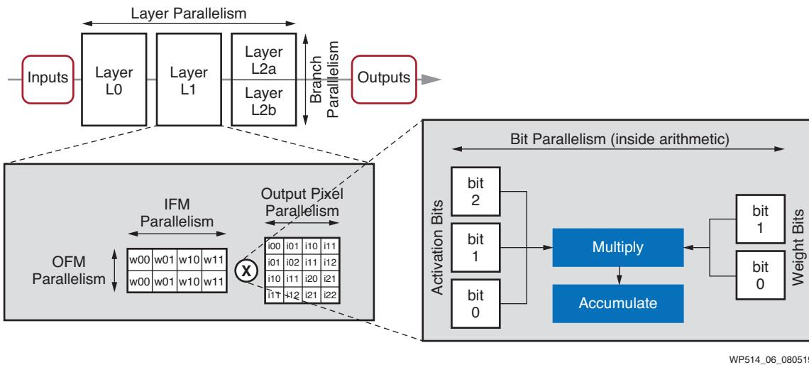
Figure 6: Levels of Parallelism Available for Computing DNN Inference
