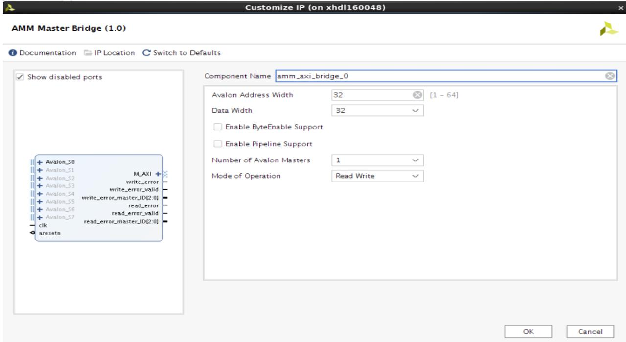
Figure 4-1: AMM Master Bridge Customize IP
