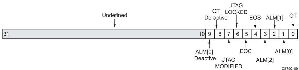
Figure 9: IP Interrupt Status Register (IPISR)
