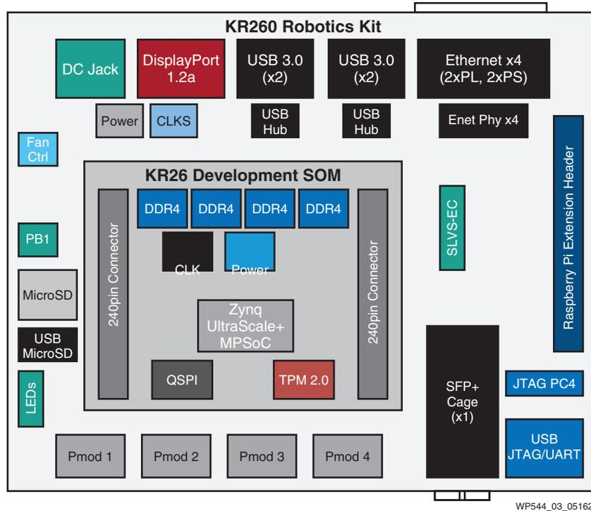
Figure 3: KR260 Starter Kit Block Diagram
