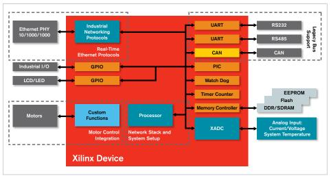
Xilinx FPGAs simplify bridging between Industrial Ethernet, traditional fieldbuses, and custom applications.
