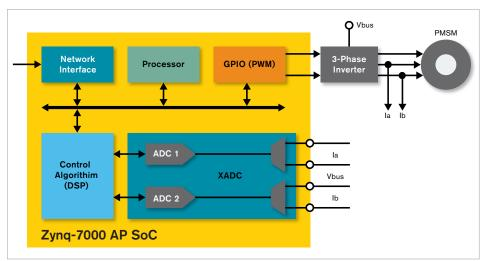
Xilinx devices enables high-performance, single-chip motor control.
