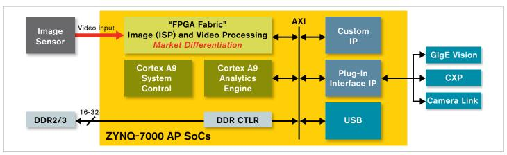
Xilinx devices are the essential components in machine vision for interfacing with sensors and transmission.
