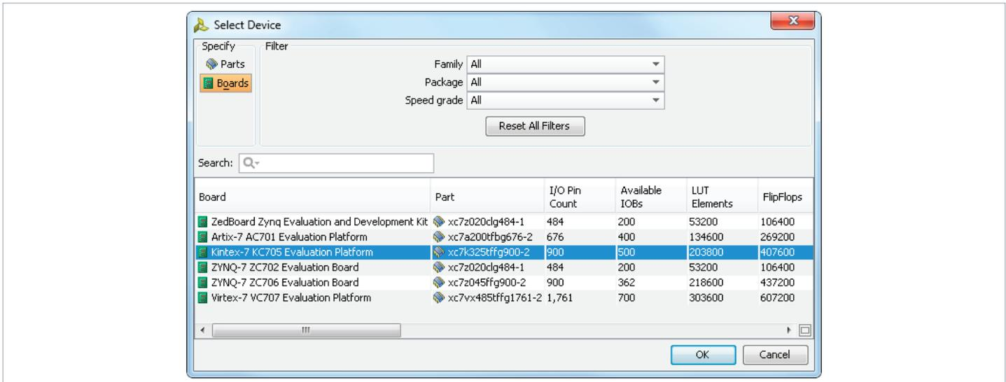
For example, by selecting the Zynq-7000 AP SoC ZC702 Evaluation Kit, and instantiating a Zynq processing system within IPI, Vivado Design Suite preconfigures the processing system with the correct peripherals, drivers, and memory map to support the board. Embedded design teams can now more rapidly identify, reuse, and integrate both software and hardware IP, targeting the dual-core ARM processing system and high-performance FPGA logic.
