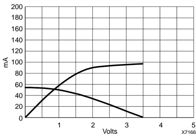
**Figure 4: Output Voltage/Current Characteristics (default for XC4000XL,**
