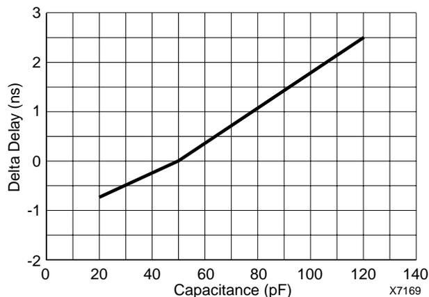
**Figure 5: Additional Delay at Various Capacitive Loads**
