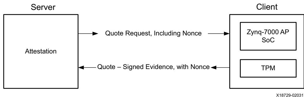
*Figure 8: Remote Attestation Using a TPM*
