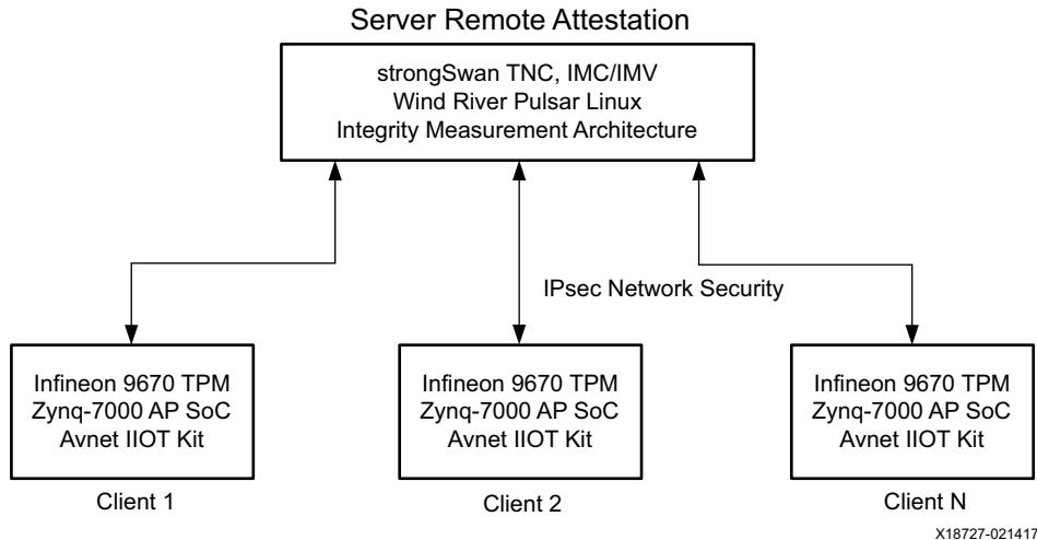
**Figure 1: Measured Boot of Zynq-7000 AP SoC Embedded Systems**
