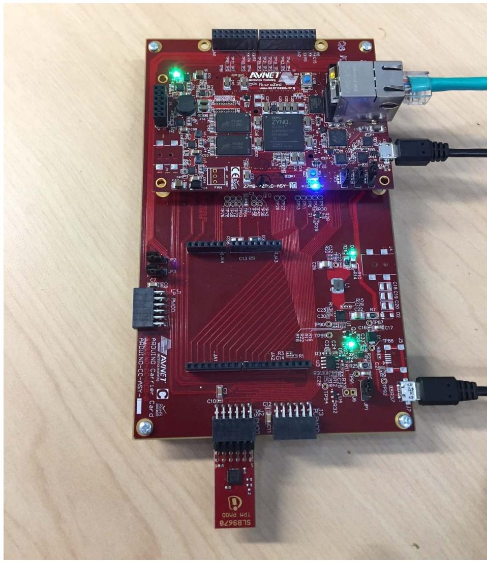
Figure 4: Avnet IIoT Starter Board with Infineon OPTIGA SLB 9670 TPM Connection
