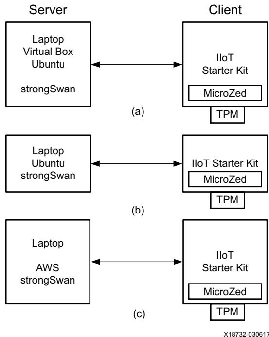
[Figure 5: Reference System Hardware Setup Options](#)
