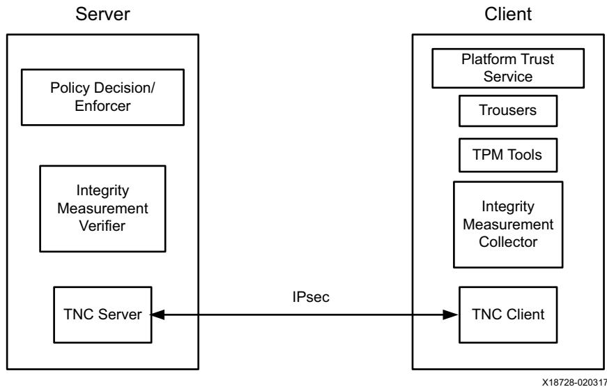
**Figure 10: Trusted Network Connect for Remote Attestation**
