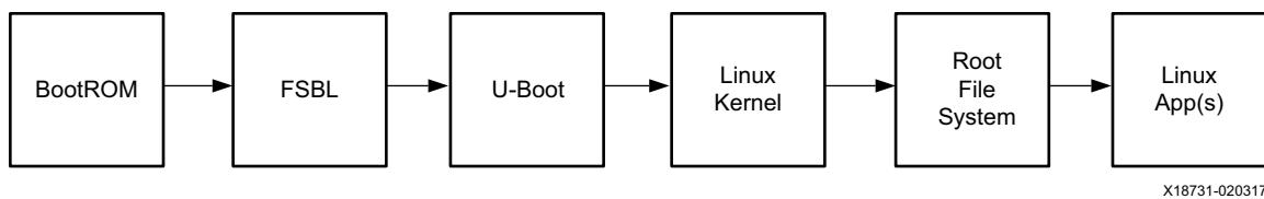
*Figure 6: Zynq-7000 AP SoC Chain of Trust Boot*
