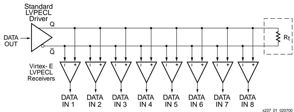
Figure 1: Typical Multi-Drop LVPECL Application
