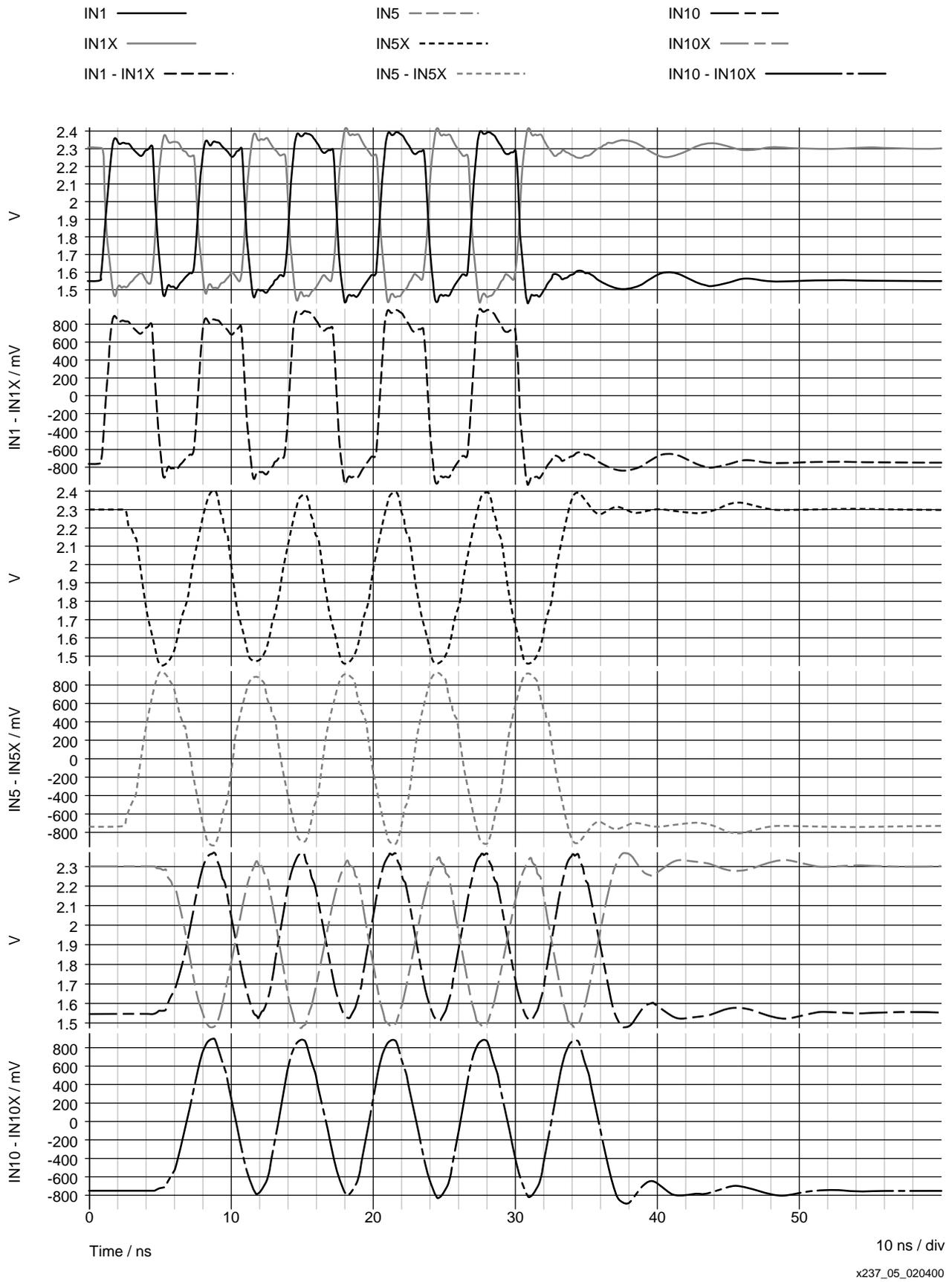
Figure 5: Typical 311 Mb/s Burst Data Response of Virtex-E Multi-Drop LVPECL Outputs.
