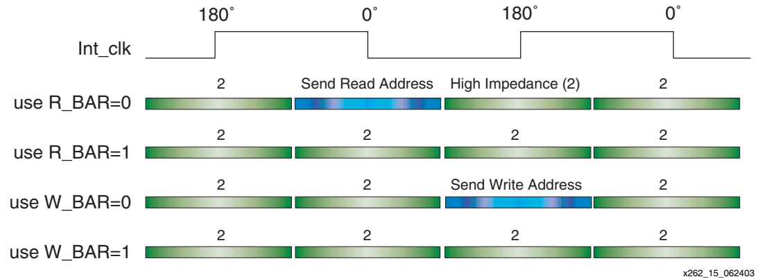
Figure 15: 2-Word Burst Address Signals
