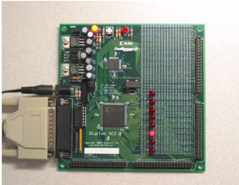
Figure 1: PicoBlaze implemented on Digilent XC2 Demoboard
