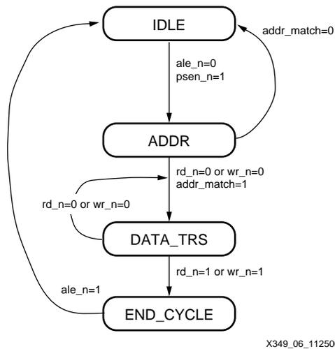
Figure 6:  $\mu$ C Bus Interface State Machine
