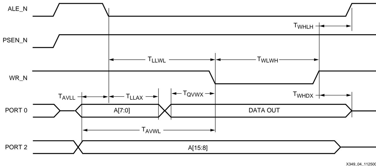
Figure 4: 8051 Microcontroller External Data Memory Write Cycle
