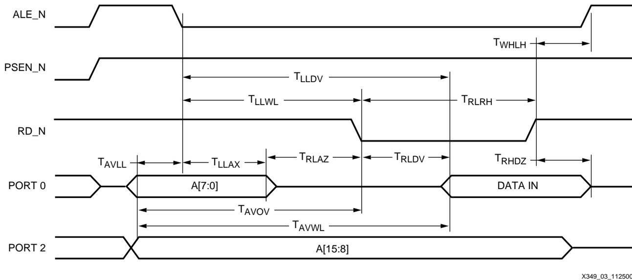
Figure 3: 8051 Microcontroller External Data Memory Read Cycle
