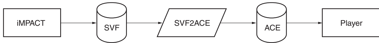
Figure 1: Design Flow For Creating and Using ACE File
