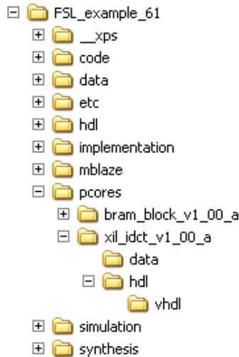
where the *xil\_idct\_v1\_00\_a/data* folder contains the MPD and the PAO file. The *vhdl* folder contains the VHDL source code of the user IP. If all the files are implemented correctly, the customized user core can be integrated in the Xilinx Platform Studio (XPS) and the bitstream of the hardware system can be generated.
