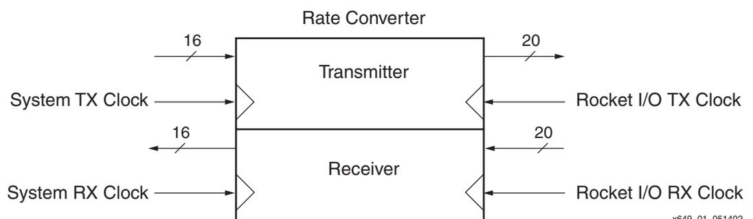
Figure 1: Rate Converter Logic Block Diagram
