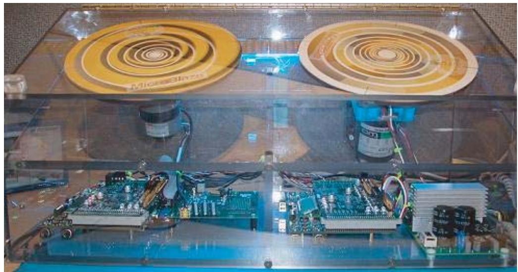
Figure 1: Motor Control Design Assembly
