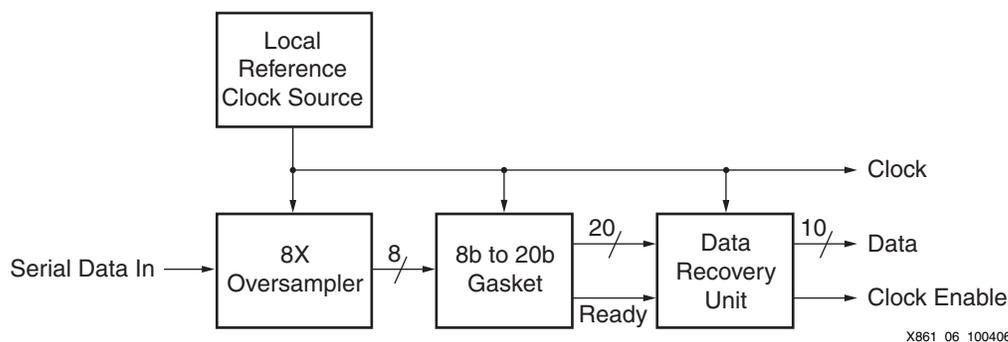
Figure 6: IDELAY-Based Oversampler with DRU
