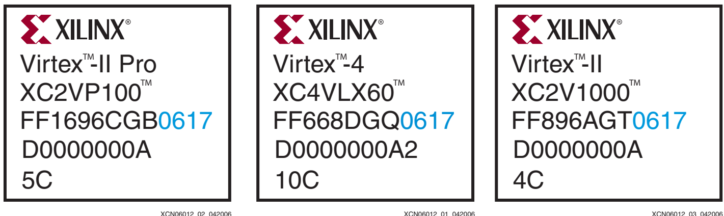
Figure 1: Virtex-II Pro, Virtex-4, and Virtex-II Package Top Marks
