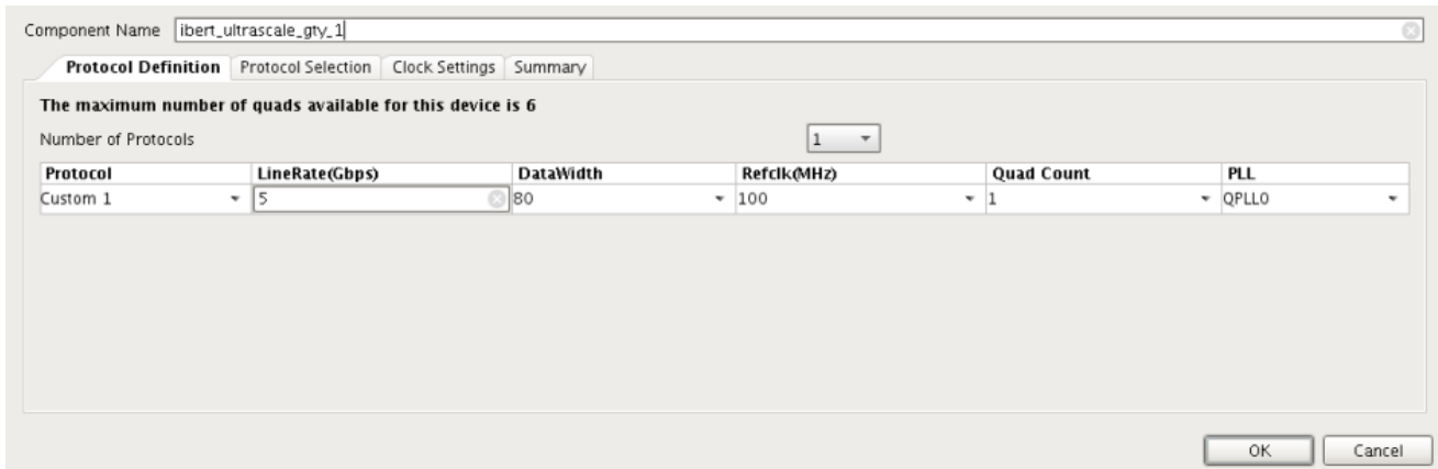
Figure 4-1: Vivado Customize IP Dialog Box – Protocol Definition
