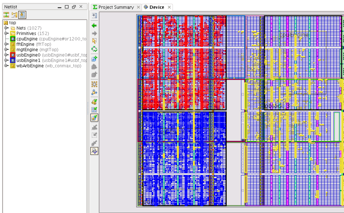
Figure 21: Implemented Design View of the usbEngine Project
