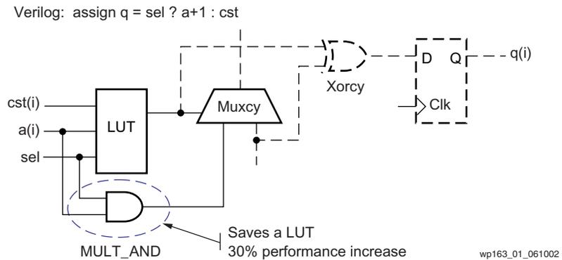
Figure 1: New and Improved Mapping for Loadable Counter
