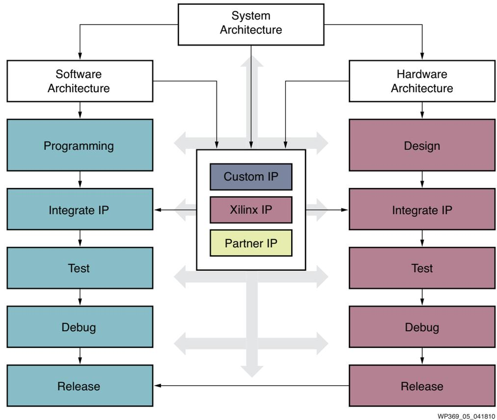
**Figure 5: Software-Centric Development Flow**
